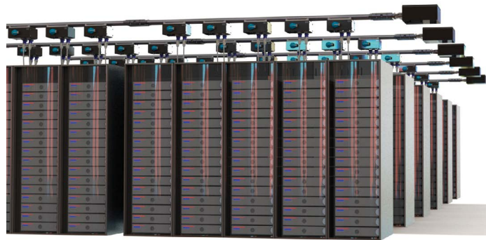
'Hot Aisle Cold Aisle' Arrangement
